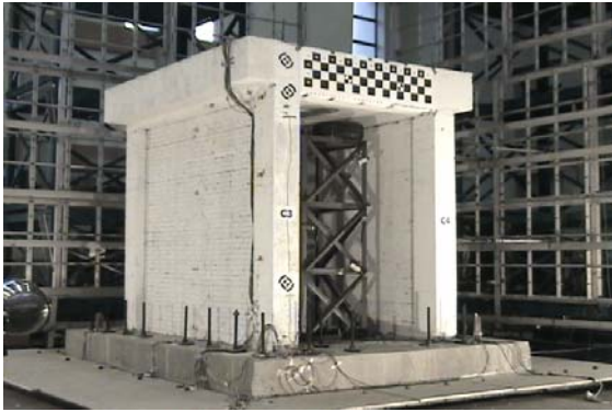
Fig. 1. Shake table test collapsing brick walls (Yuan-Sen Yang, E-mail: ysyang@ncree.org.tw)
